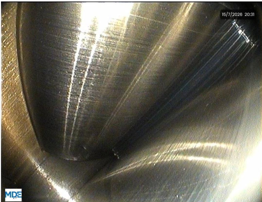
Photo 2: Bearing input shaft, mid, driven end. No deviations have been observed.
