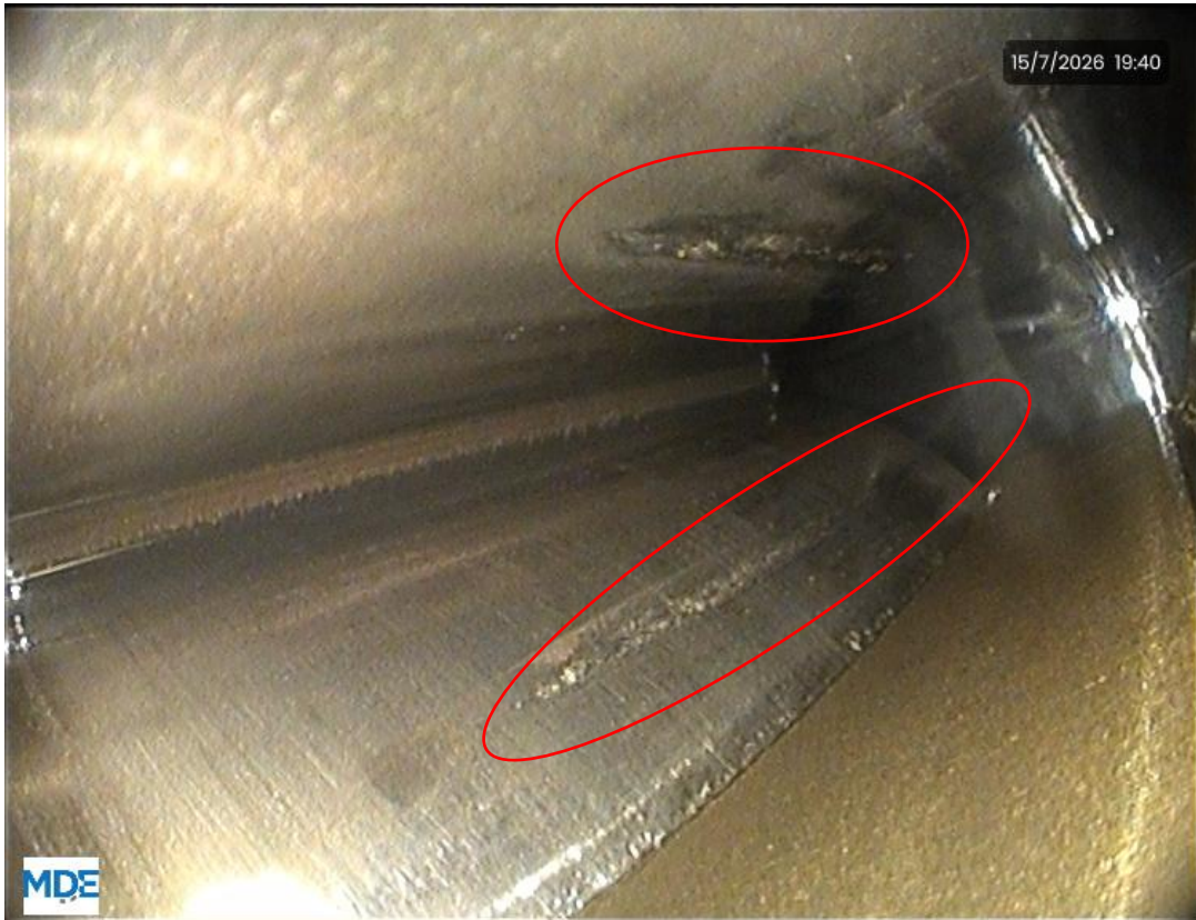
Photo 9: PTO mid, mid, non-driven end. Pitting, false brinelling have been observed.
