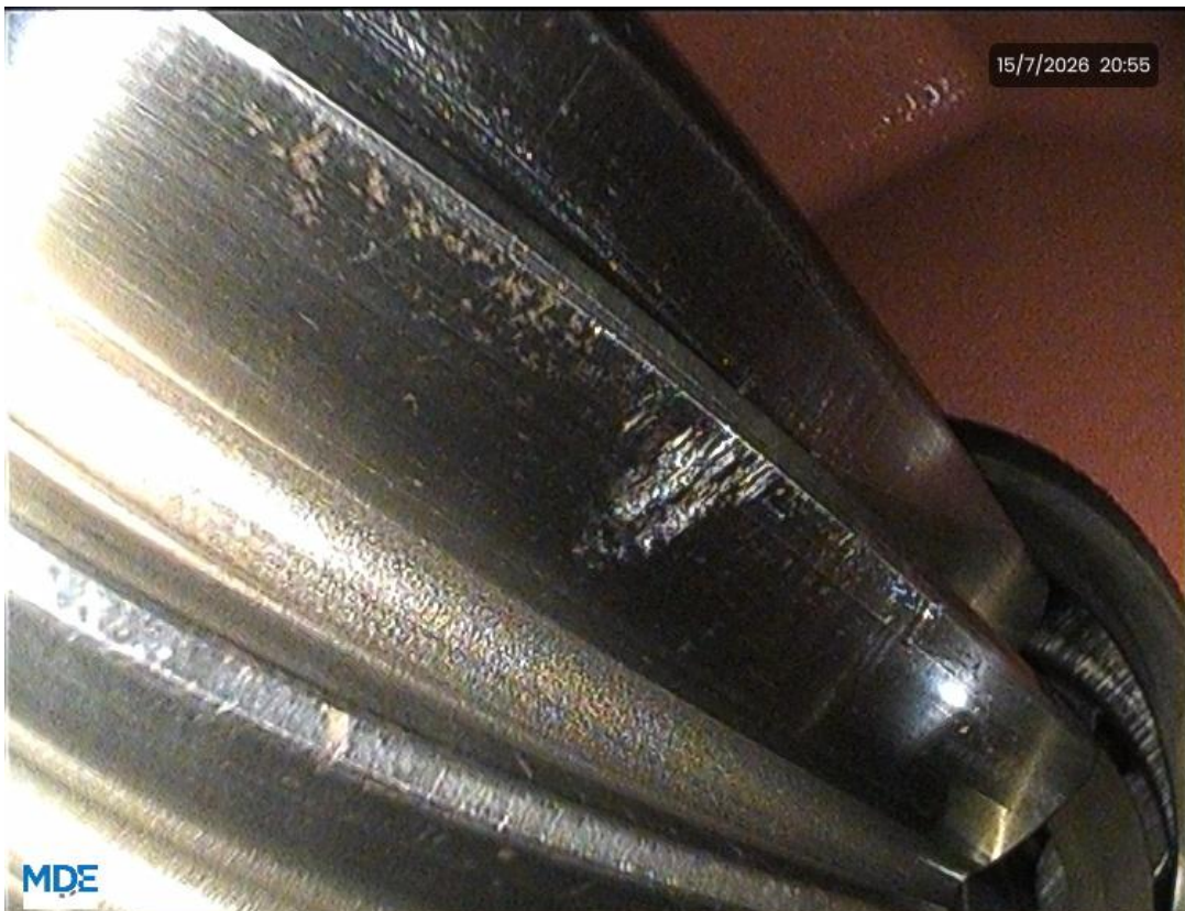
Photo 4: PTO pinion. Minor corrosion and minor scuffing have been observed.
