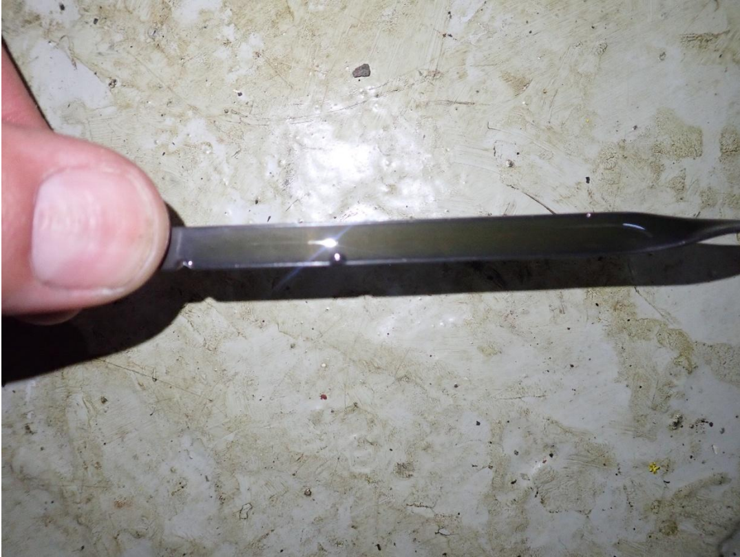
Photo 1: Dipstick. Oil is on the prescribed level.
