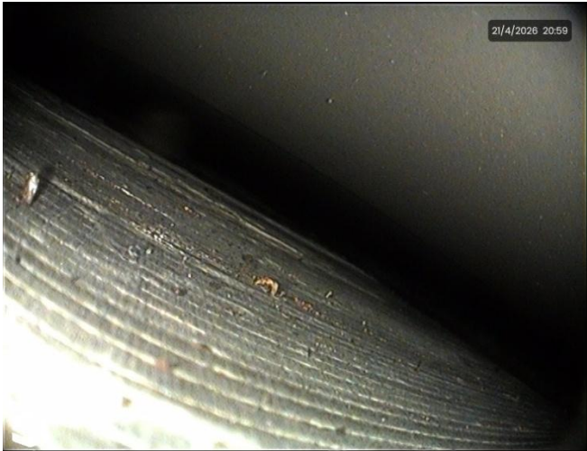
Photo 25: Coil 46. Debris and paint damage
